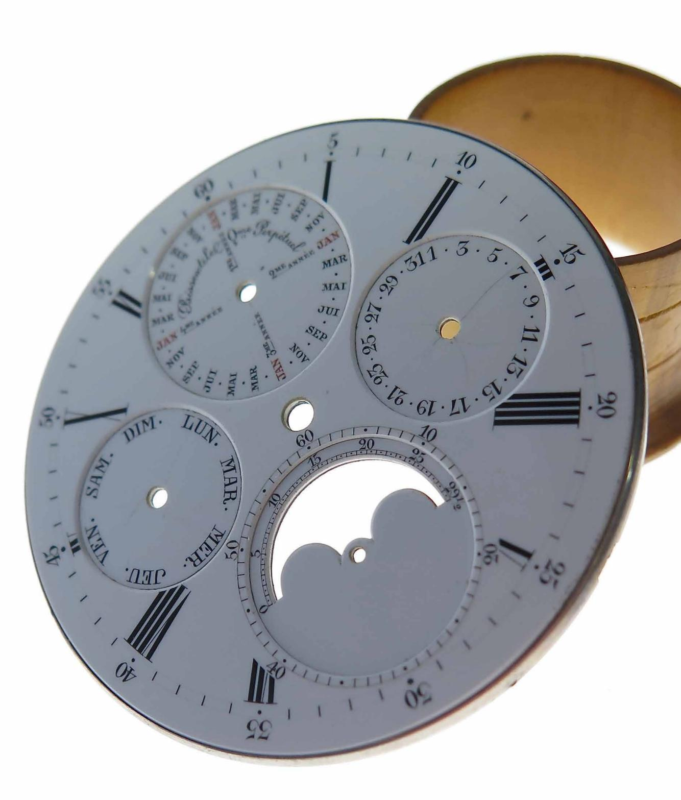
The dial removed from the case and movement. The fine, hair line fractures in the subsiduary dials are probably the result of the subsiduary hands being removed at somepoint during the watches life.
